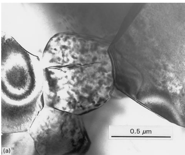
Figure 4 Micrographs showing the variation of sizes of order domains in BZN13: (a) apparent influence of grain size, (b) apparent influence of migration of grain boundaries and earlier presence of fine-grained particulate.
