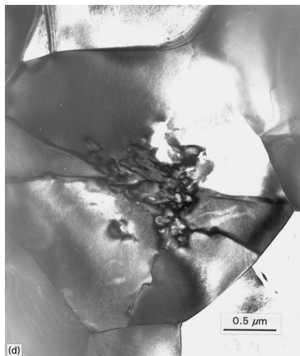
Figure 11 Micrographs showing (a) a pocket of unsintered mixed powder grains in BZN13, (b) a dislocation that has climbed and dissociated in a grain of BZN15, (c) the stacking fault contrast of another dislocation in BZN15 that has climbed and dissociated, (d) a typical core/shell grain microstructure in BMT16.
