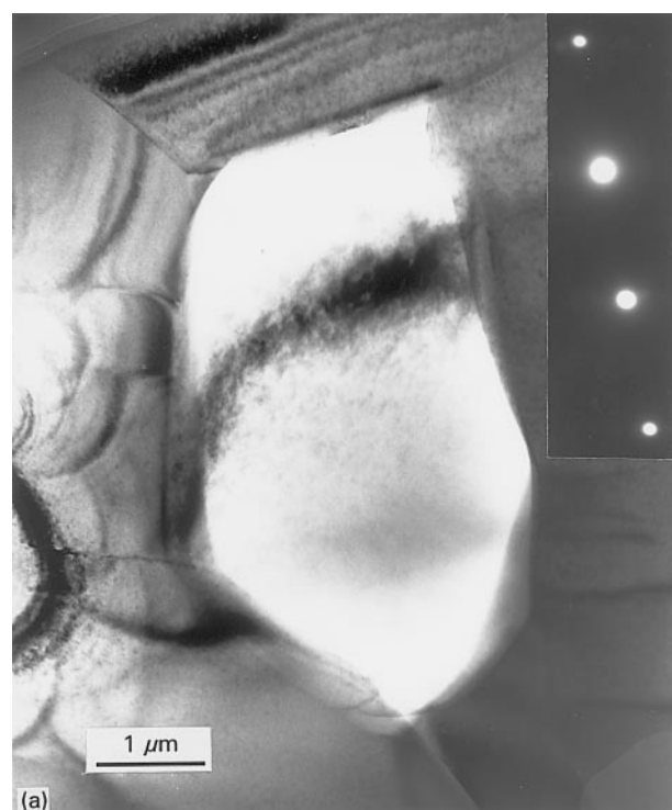
Figure 7 (a) Micrograph of an MgO grain in BMT16 with SAD (inset) and (b) EDX microanalysis spectrum from the grain.
