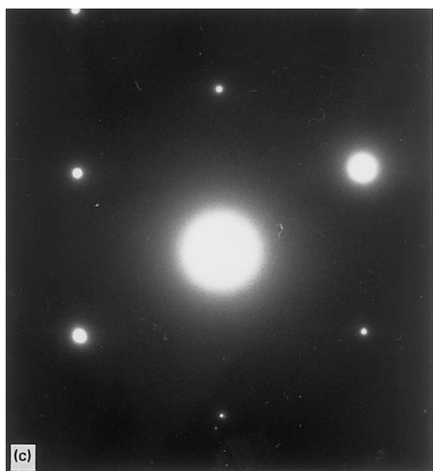
Figure 10 Dark-field micrograph taken with a superlattice reflection showing large 1:2 ordered domains adjacent to a grain boundary in BZT15, (b) micrograph showing a region containing domains of 1:1 order adjacent to a dislocation within a grain which has predominantly 1:2 order, (c) SAD from the 1:1 ordered region, (d) SAD from the 1:2 ordered area surrounding the 1:1 region, (e) micrograph showing a region with anomalously large 1:2 domains and which contains a wall of dislocations in BZT15 (the dislocations are slightly inclined to the electron beam where there are several arrows, and parallel to it where there is a single arrow).
